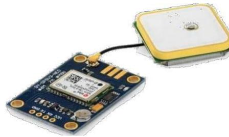
Figure 5: Global Positioning System Module
